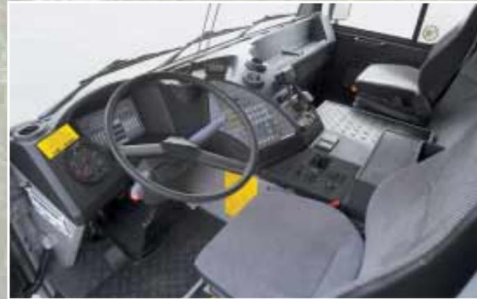
The elevating crane cabin has continuous height adjustment to ensure optimum visibility. The Electronic Monitoring System (EMS) gives the crane operator a full view of all crane functions.
