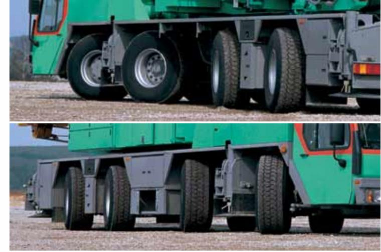
The four steered axles ensure optimum manoeuvrability.
