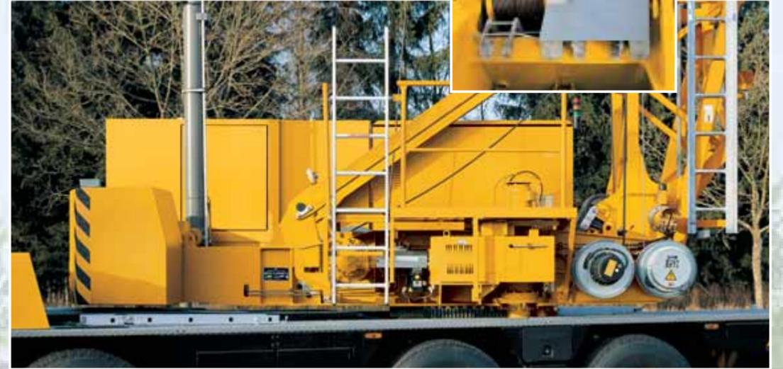
On the superstructure, all drives are integrated. They feature frequency converter control and thus provide continuously variable speeds. EDC slewing gear is fitted with an electronic control system and also offers continuously variable working speeds, with electronic wind-load compensation, automatic anti-swing load damping and safe counter-current capability. The MK 80 features complete ballast as standard equipment, and an integral generator.
